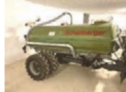
Schallberger 3000 Lt. Pumpe 10 Bar 75 m 3 , el. Turm
