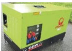
**Pramac GBW22Y Generator, neu, Notstromleistung LTP 15.2 kW, 19 kVA, 400V/230V, Dieselmotor Yanmar, 560 kg**
